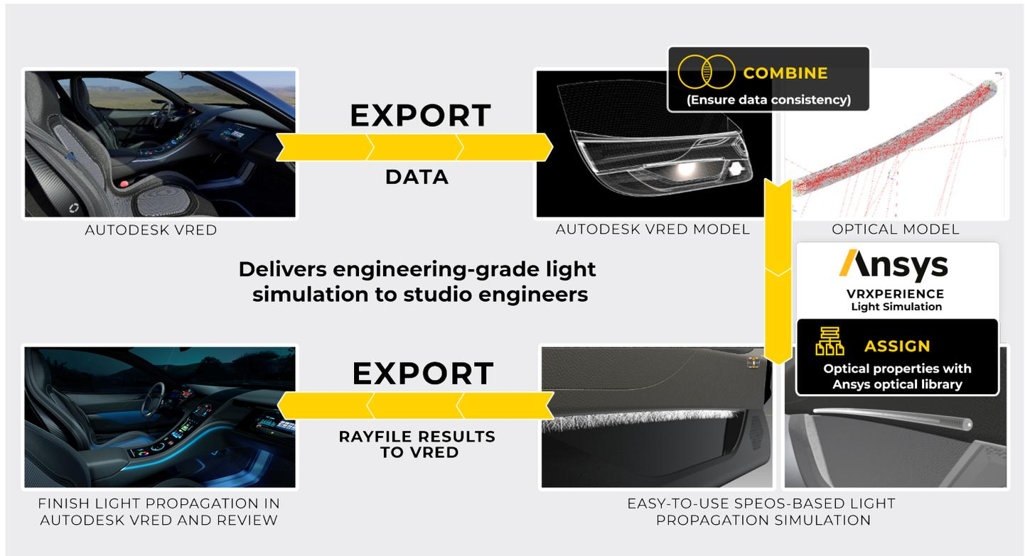
The workflow detects defects such as lighting uniformity or light leakage that cannot be discovered without optical simulations and validates lighting appearance design intent.
